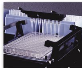
8-channel pipettor accessing a 96-well microplate
